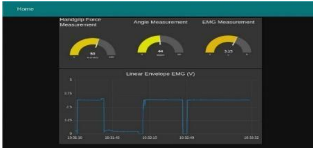
Fig. 5. The IoT architecture; a) four layers of IoT architecture, b) dashboard created using Node-Red.
